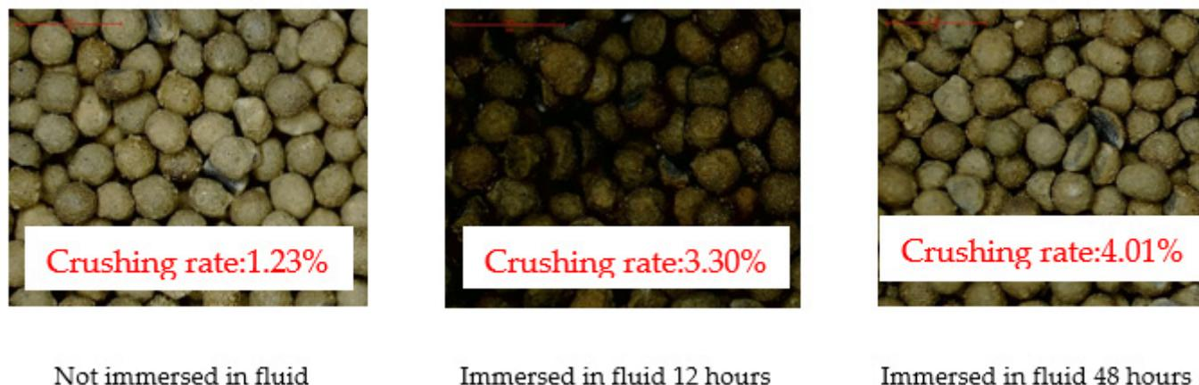
Figure 5. Proppant crushing test results.
