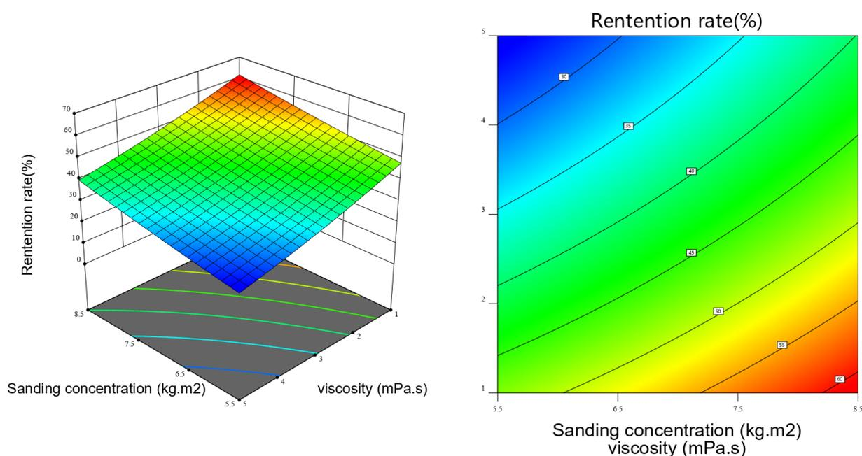
**Figure 6.** Response surface and contour plots (sand concentration vs. viscosity).
