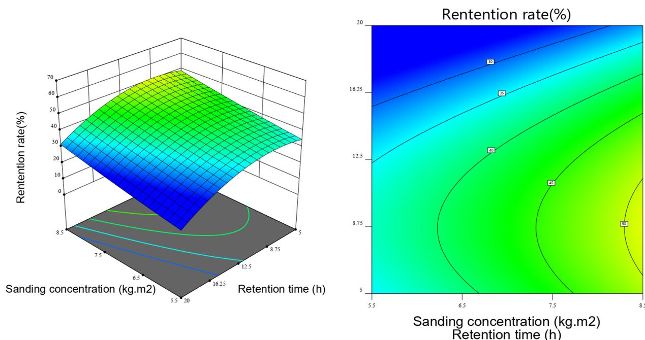
**Figure 7.** Response surface and contour plots (sand concentration vs. retention time).
