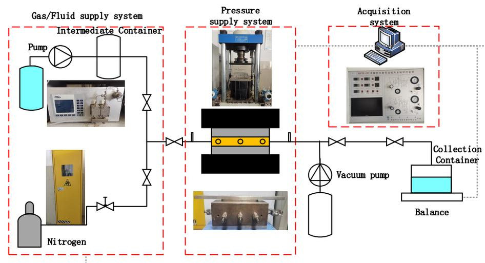
Figure 1. Flow conductivity damage test procedure.
