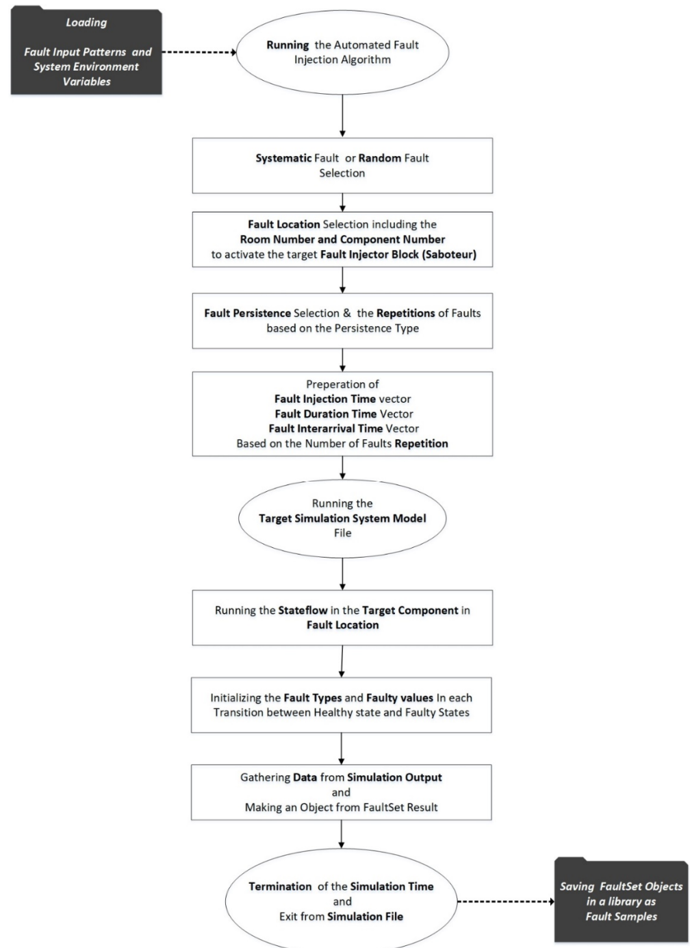
Figure 6. Steps of implementation of the automated fault injection process using Stateflow diagram.
