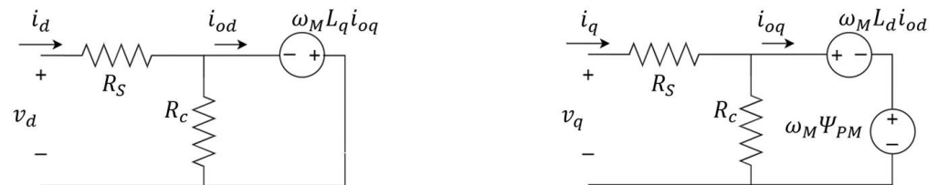
Figure 9. Synchronous machine equivalent circuit considering core-losses on a d - q reference frame.
