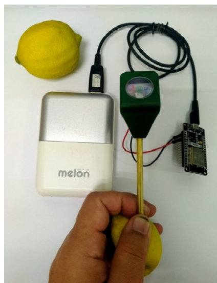
Figure 10. Testing of pH measurements with a proposed device when working with small uninterruptible power supplies.
