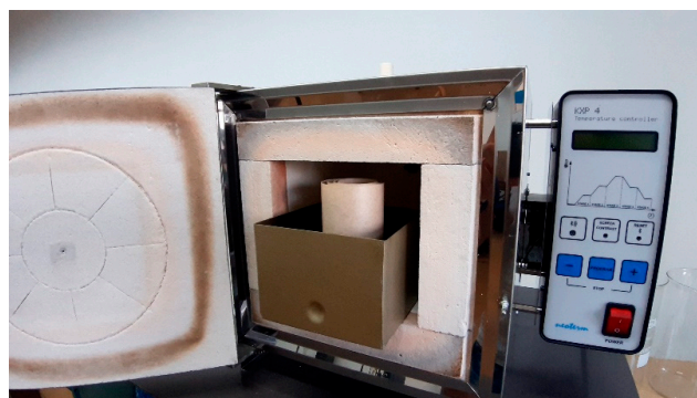
Figure 5. System to perform the accelerated ageing process of the NOMEX ® 910 insulation samples.
