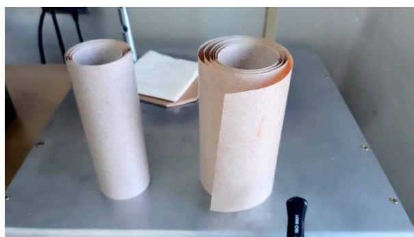
Figure 2. Test samples of the NOMEX ® 910 insulating material prior to impregnation.
