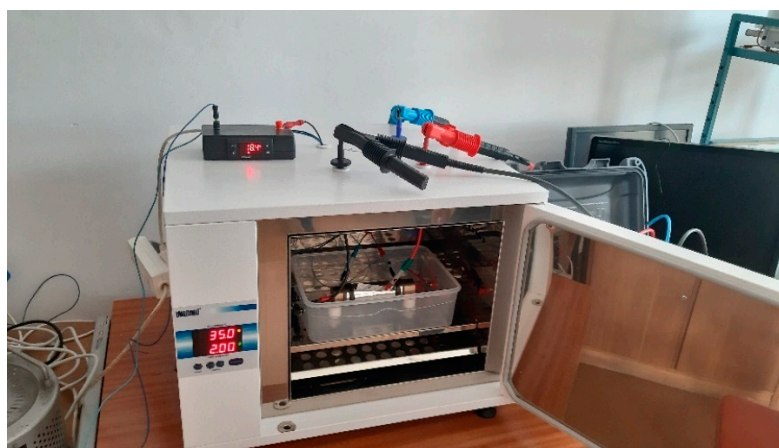
Figure 8. Laboratory station for measuring polarization and depolarization currents in transformer insulation samples with the ambient temperature stabilizer visible.
