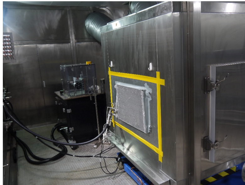
Figure 5. The heat exchanger performance test platform.
