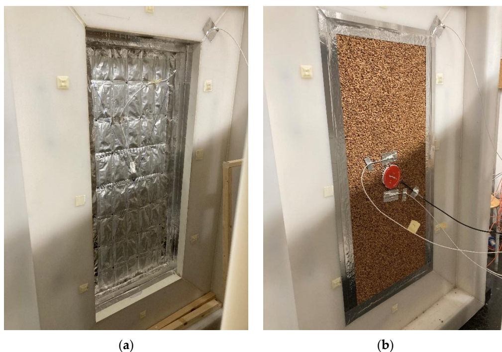
Figure 23. Details of the installation of the PCM sheet inside the SuberWall panel sample (a) and the probes used for the monitoring of the main thermal characteristics (b) by a climatic chamber.
