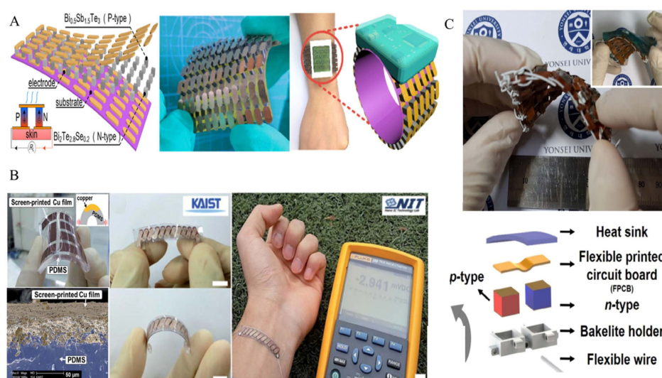
Figure 5. (A) Structural design and fabricated images of ns-FTEGs and FTEGs-powered wearable multi-sensory bracelet [49]. (B) Schematic illustration of the flexibility of the embedded Cu film (Cu foil vs. the screen-printed Cu film) in PDMS and demonstration of band-type flexible TE generator for harvesting thermal energy from human skin at an air temperature of 15 ^{\circ}\text{C} (scale bar, 1 cm) [50]. (C) Schematic design and structure of ns-FTEGs encapsulated by bakelite [51].
