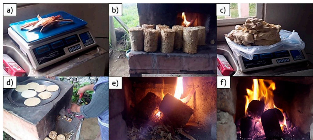
Figure 4. (a) Firestarter (weight), (b) Briquettes (biofuel), (c) Tortilla dough (weight), (d) Field cooking in the Patsari cookstove, (e) Combustion during the starting of the cooking test, (f) Generation of charcoal before finishing the test.
