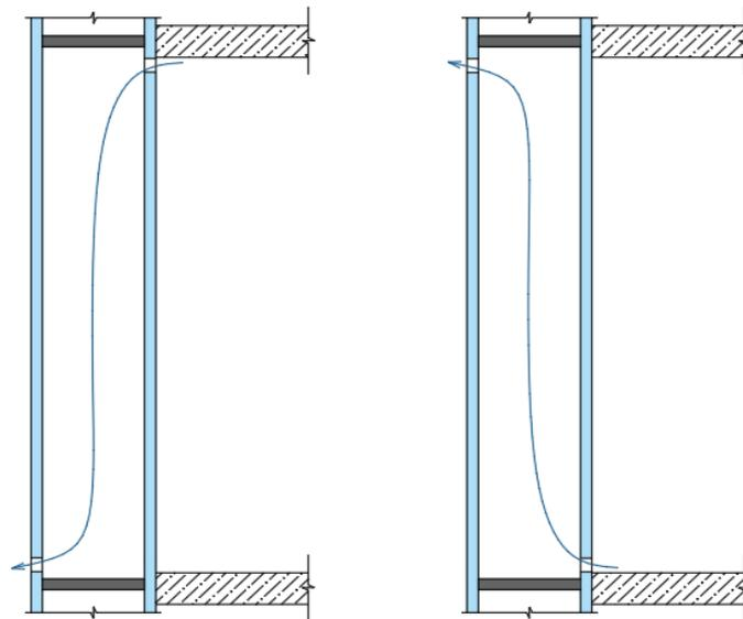
**Figure 12.** Facade systems with exhaust mode.
