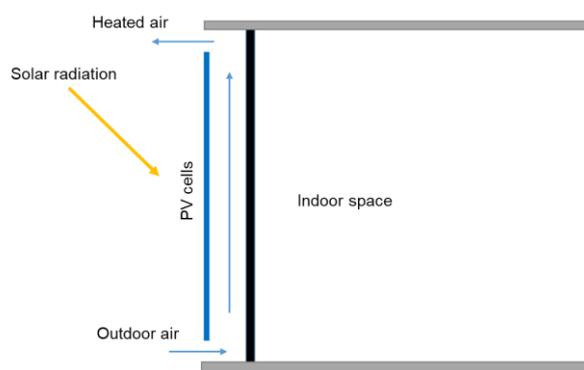
**Figure 15.** Scheme of ventilated passive PV facade.
