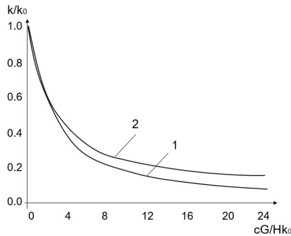
Figure 19. Relative heat transfer coefficient of the ventilated facade: 1—double glazing, 2—triple glazing.
