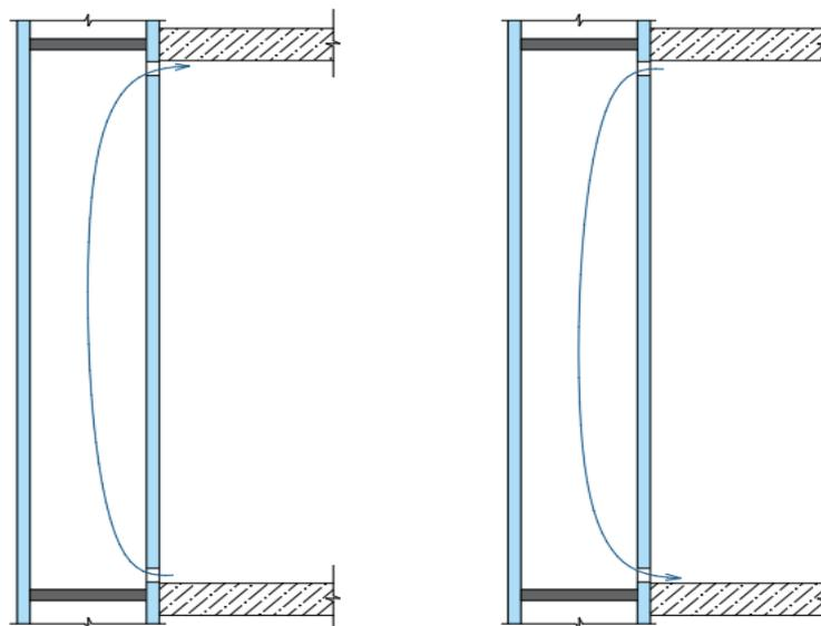
**Figure 9.** Facade systems with ventilation of the interstitial space with internal air (internal air curtain).
