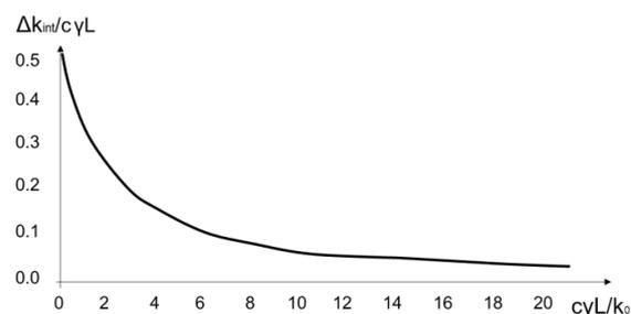
**Figure 21.** Dimensionless increment of the heat transfer coefficient of a ventilated facade with triple glazing.
