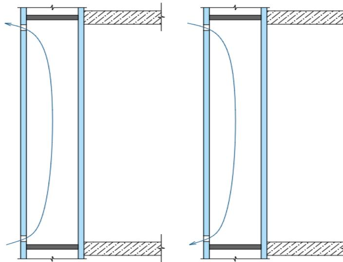
**Figure 10.** Facades with ventilated air gap by external air (external air curtain).
