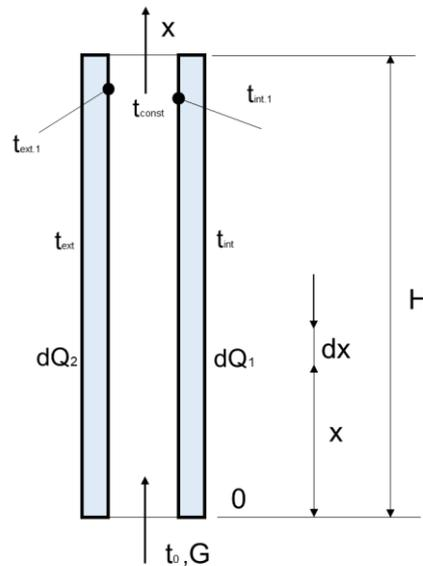
**Figure 18.** Scheme of a ventilated facade for calculation using the heat balance equation in a ventilated layer.
