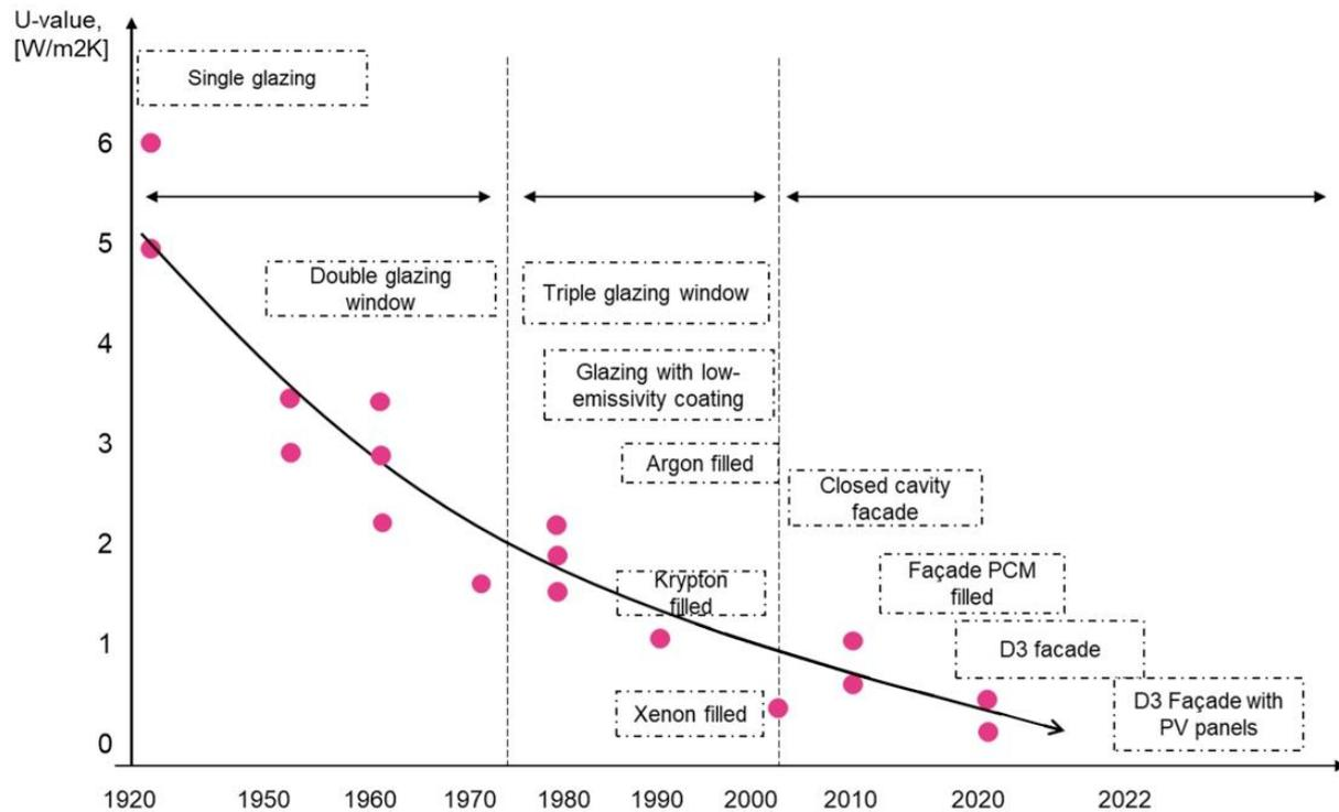
**Figure 1.** Development U-value of window and glazing façade.
