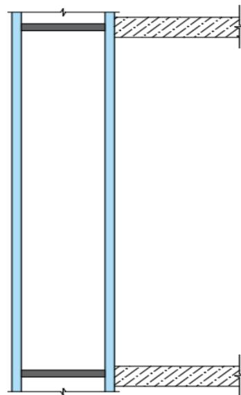
**Figure 13.** Facade systems with closed air layers (buffer zones).
