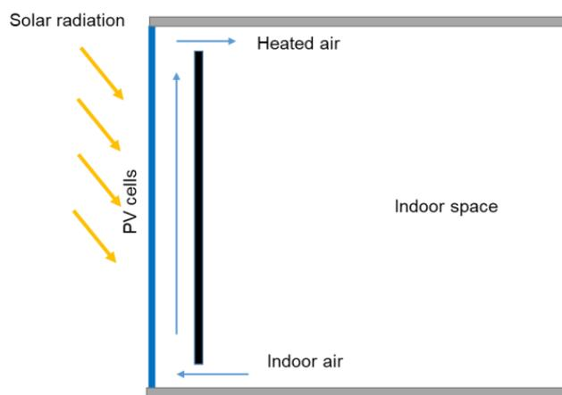
**Figure 16.** Scheme of ventilated active PV facade.
