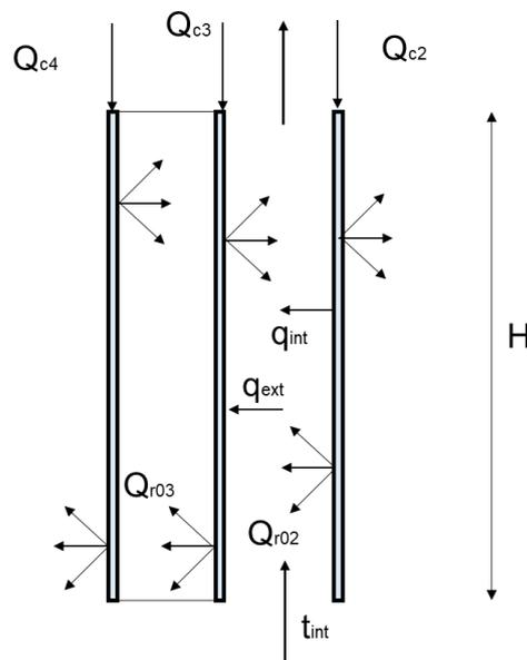
Figure 20. Scheme of a ventilated facade for calculation according to the heat balance equations on glass surfaces.
