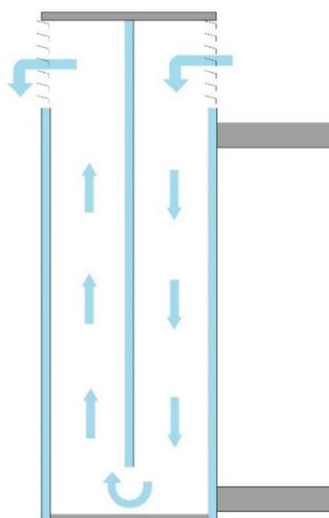
**Figure 14.** Triple ventilated facade with U-shaped airflow.
