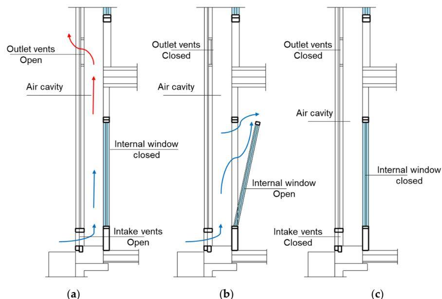
Figure 17. Adaptive ventilated facades with controlled thermal characteristics. (a) summer daytime, (b) summer night, (c) winter.
