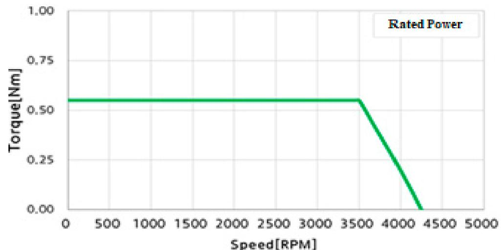
**Figure 2.** Torque-Nominal Speed curve of the target model.
