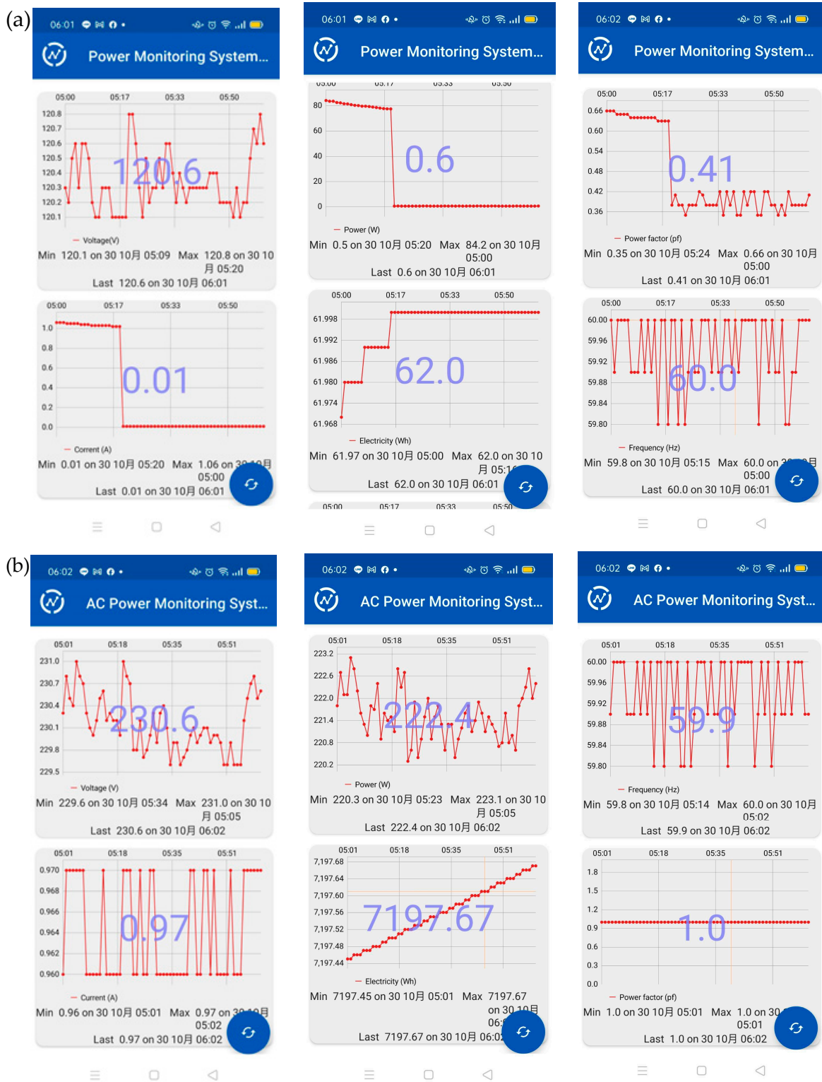
Figure 10. Parameter visualization of voltage, current, electrical power and energy, pf, and frequency in the ThingView: (a) Refrigerator; (b) Air conditioner.
