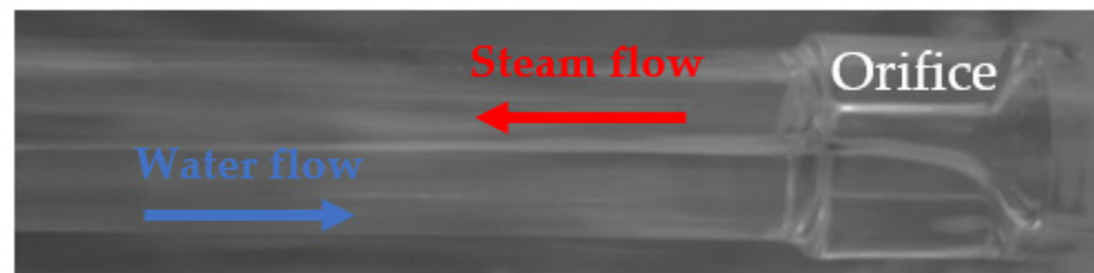
Figure 8. Countercurrent flow in the orifice.
