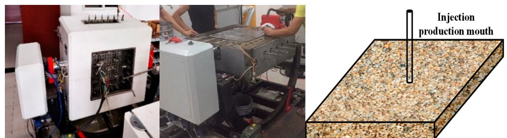
Figure 2. Two-dimensional core simulation setup: (left) overall appearance; (middle) plate placement, (right) schematic diagram of the injection and mining method.
