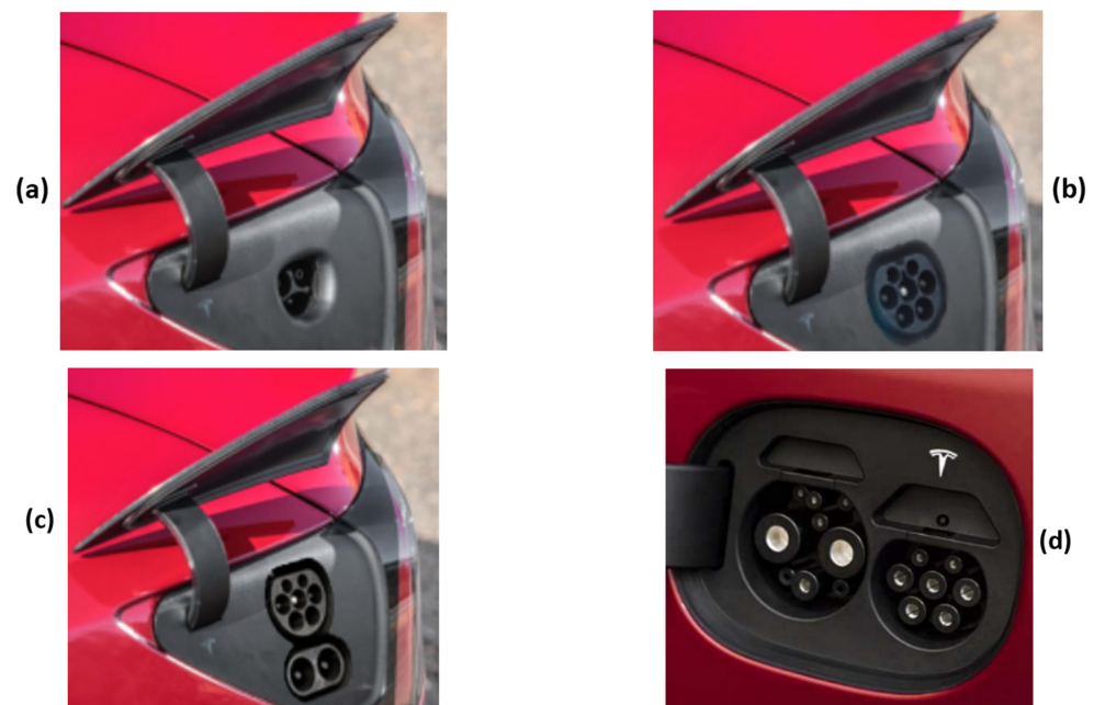
Figure 27. The Tesla EV inlet according to the region of sale: (a) US; (b) and (c) EU; (d) China.
