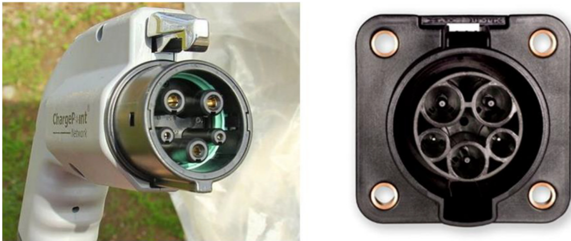
Figure 11. The SAE J1772 EV charging coupler: EV Plug (Left) and Inlet (Right).
