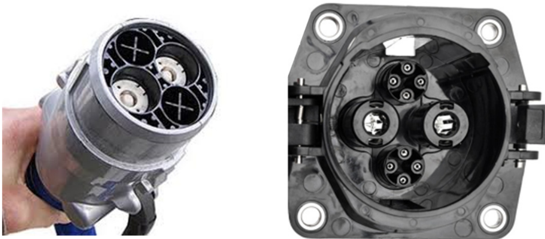
Figure 17. The CHAdeMO coupler: EV Plug (Left) and Inlet (Right).
