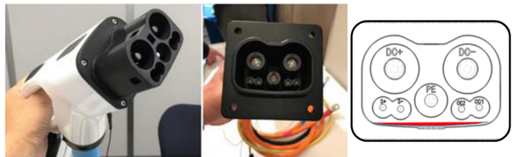
Figure 25. The Chaoji coupler: EV Plug (Left), Inlet (Middle), and Inlet pinout (Right).
