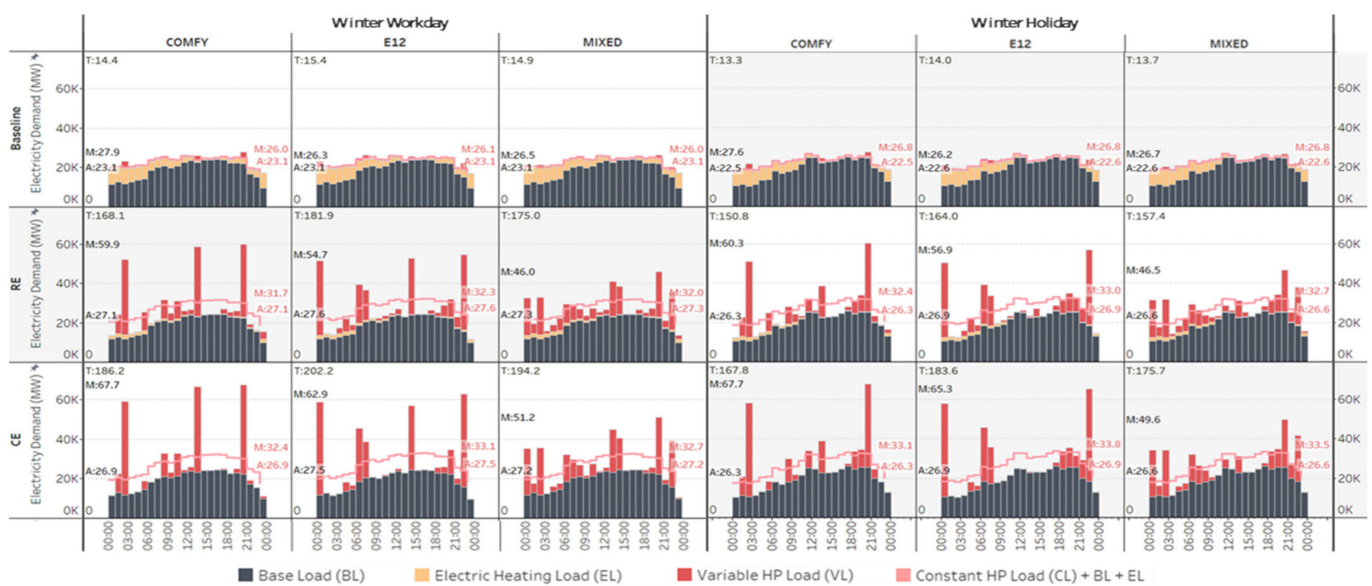
Figure 17. Average hourly electricity demand load curve of heat pump scenarios for Orkney for the coldest winter workday and holiday (T: Total, M: Maximum, A: Average).
