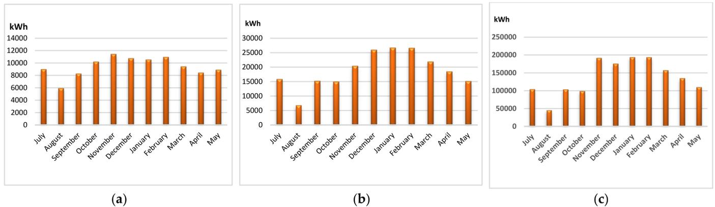
**Figure 1.** Average monthly consumption of a: (a) 5.7 kW consumer, (b) 12 kW consumer, and (c) 15 kW consumer.
