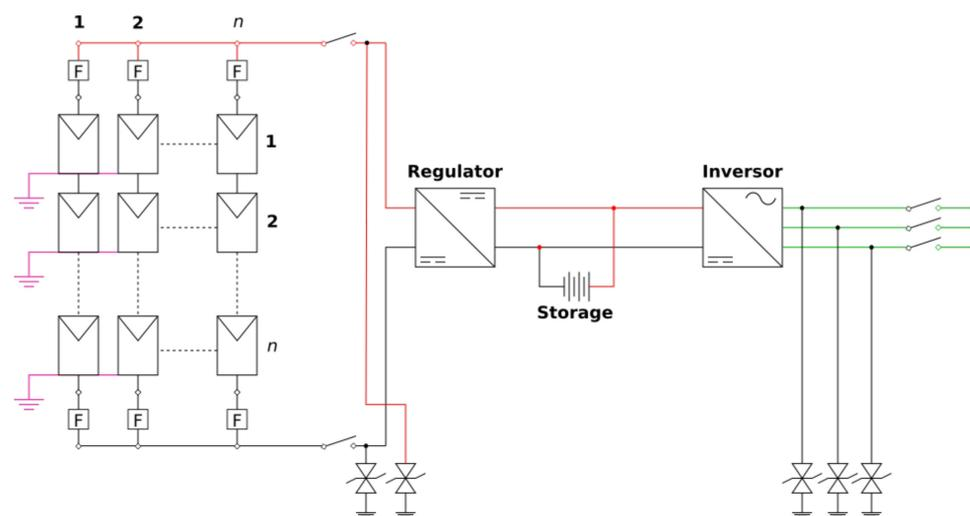
Figure 7. General electrical diagram of the photovoltaic installation.
