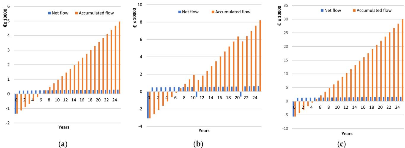
Figure 8. Cash flow for a physical LEC: (a) alternative 1, with no batteries and no incentives, (b) alternative 2, with batteries and no incentives, and (c) alternative 3, with no batteries and no incentives.
