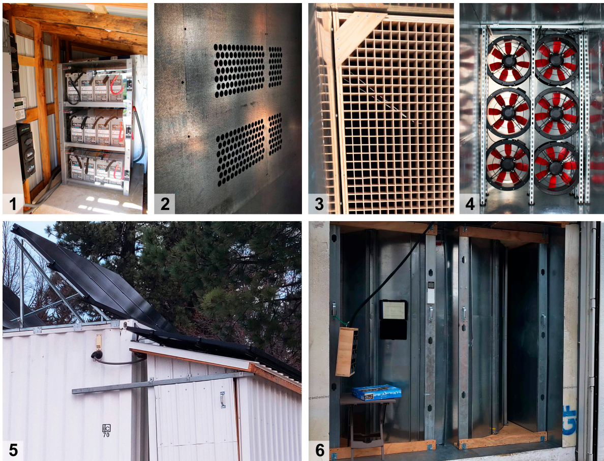
Figure 6. Test chamber construction photos. (1) Battery rack in doghouse. (2) Perforated access panel for mini-split indoor unit. (3) Air straightener placed in chamber test side. (4) Fan array fixed in place. (5) Weather-proof port connecting doghouse to chamber. (6) Door-side corner fairings.
