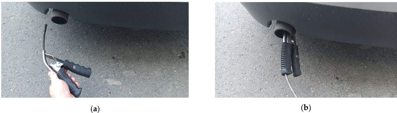
Figure 2. Measurement probe: (a) exhaust emission measurement probe during assembly; (b) measuring probe placed in the vehicle's exhaust system.
