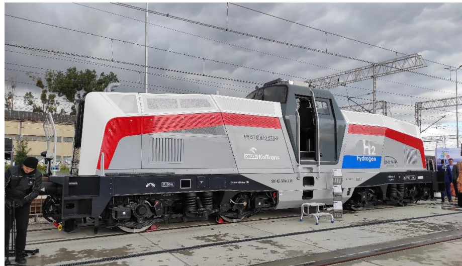
Figure 16. The hit of Trako 2021. PESA presented a hydrogen locomotive based on the SM42 [photo by Jaroslaw Konieczny].
