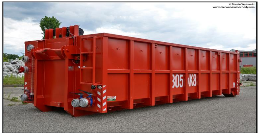
Figure 14. A container for extinguishing electric vehicles, manufactured by Ekombud, belonging to JRG-5 Kraków [55].
