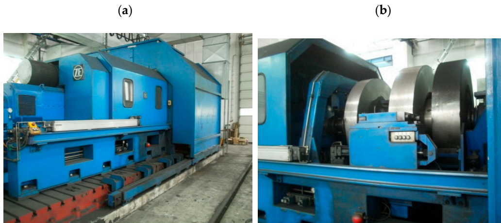
Figure 5. Test stand: (a) general view, (b) mechanical flywheels.
