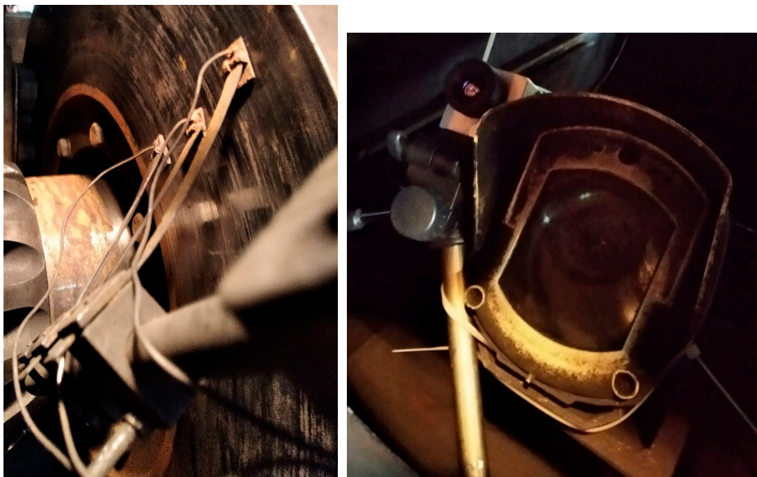
Figure 6. Research object, slip thermocouples and infrared camera.
