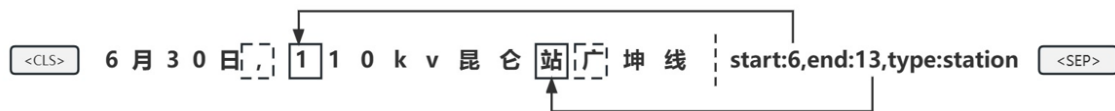
Figure 4. “6月30日, 110 kV 昆仑站广坤线” corresponds to “On 30 June, 110 kV Kunlun Station Guangkun Line”. Deep contextual semantic information. The solid line matrix box represents the character information corresponding to the start and end positions of the candidate span in the text, and the dashed matrix box represents the character information corresponding to one offset before and after the start and end positions of the candidate span in the text.
