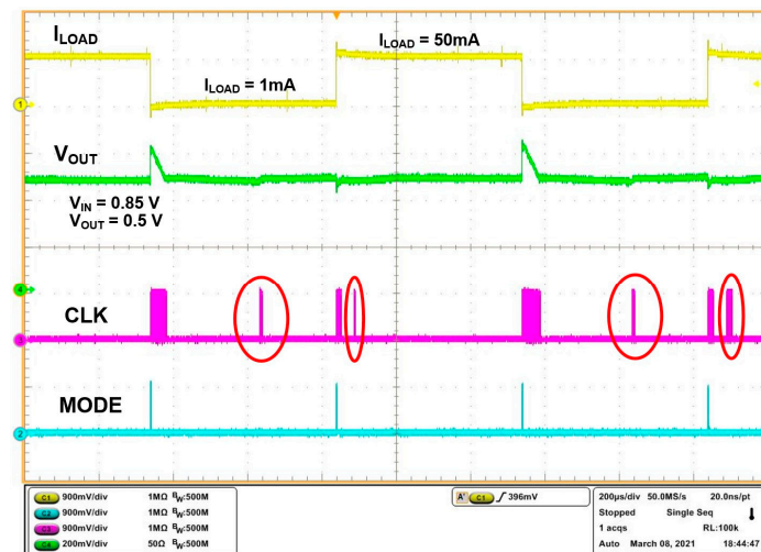
Figure 15. Transient waveforms of V_{OUT} clamping by the window of V_{REF\_L} and V_{REF\_H} .
