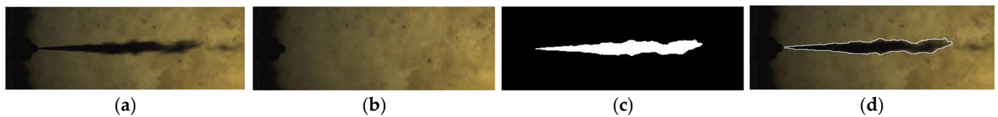
Figure 4. Image processing sequence for liquid boundary detection. (a) Raw image; (b) Background image; (c) Binary image; (d) Determined boundary.
