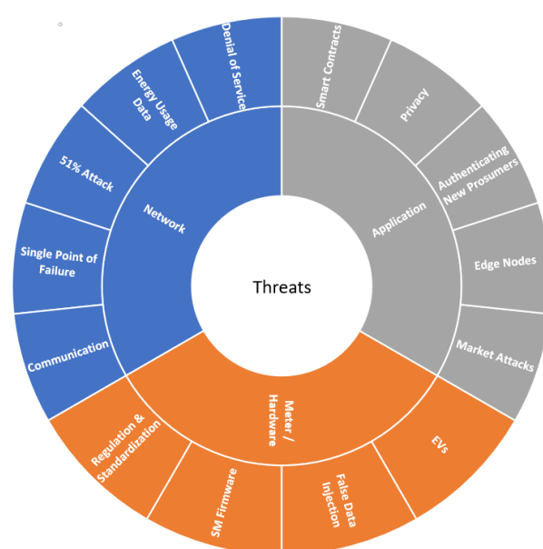
Figure 1. Simple taxonomy of the threats discovered. There are three overarching categories; the application layer, the network layer, and the hardware layer (including the smart meter itself). Each threat is relevant to at least one of these categories.
