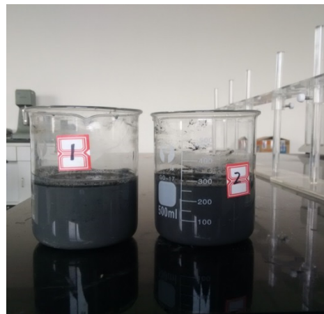
Figure 2. Picture of oily sludge profile control system prepared in the laboratory.
