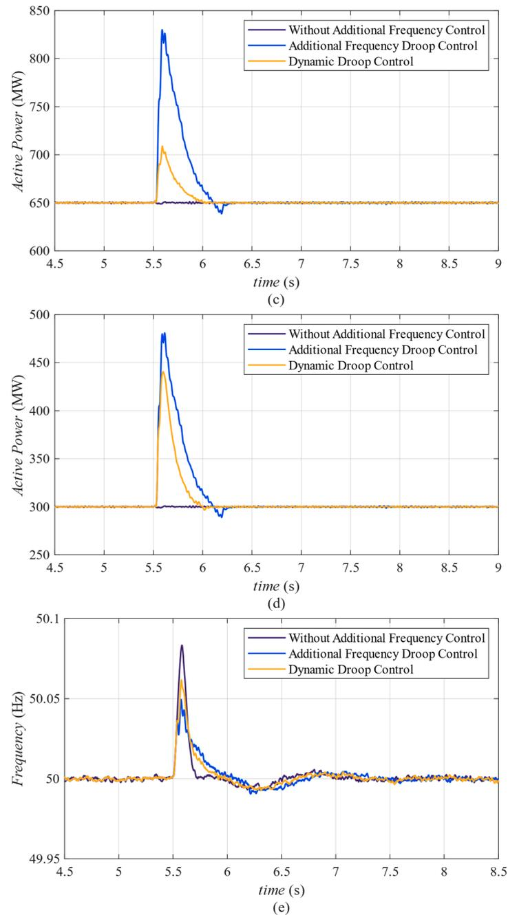
**Figure 8.** System response when wind power generation increased; (a) active power of line 1; (b) active power of line 2; (c) active power of line 3; (d) active power of line 4; (e) system frequency.
