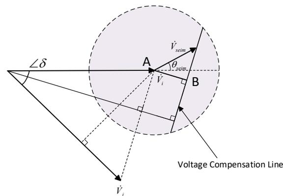
**Figure 3.** Illustration of voltage compensation line.
