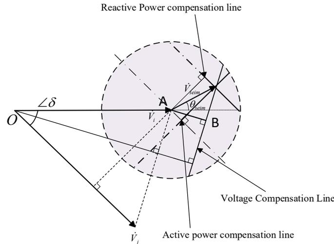
Figure 4. Vector diagram for IPFC.
