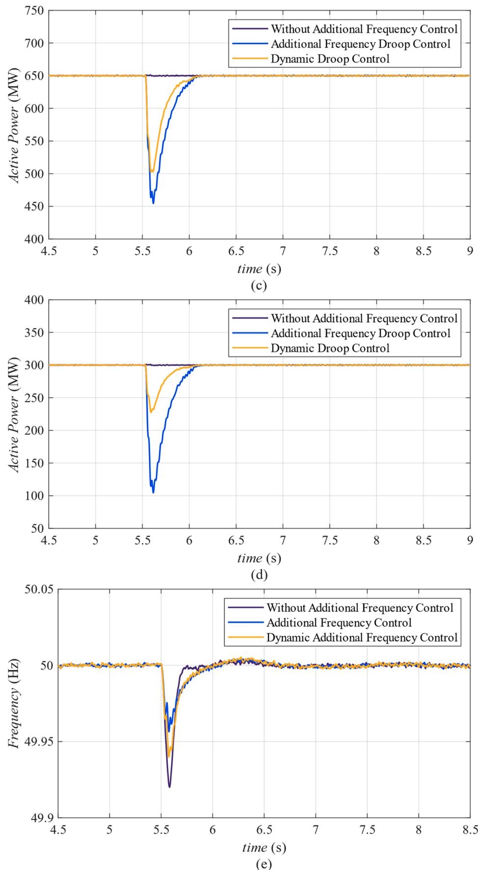
**Figure 9.** System response when wind power generation decreased; (a) active power of line 1; (b) active power of line 3; (c) active power of line 4; (d) active power of line 4; (e) system frequency.
