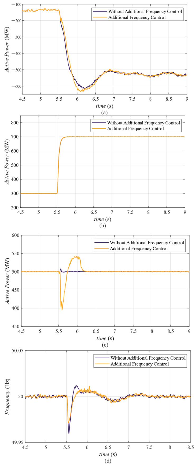
**Figure 6.** System response when line load increased. (a) Active power of line 1; (b) active power of line 3; (c) active power of line 4; (d) system frequency.
