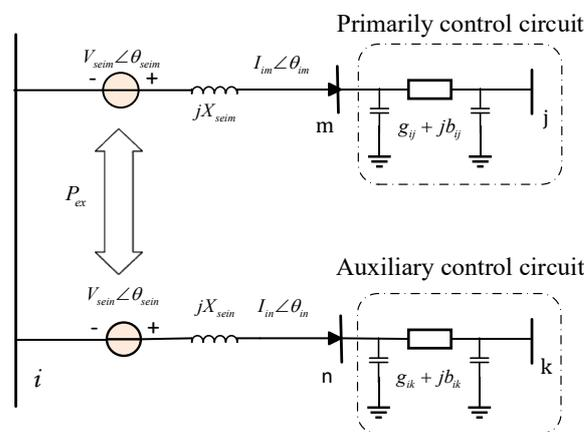
Figure 2. An equivalent circuit diagram of the IPFC.
