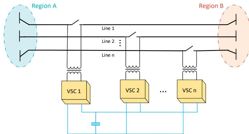
Figure 1. A simplified structure diagram of an IPFC.
