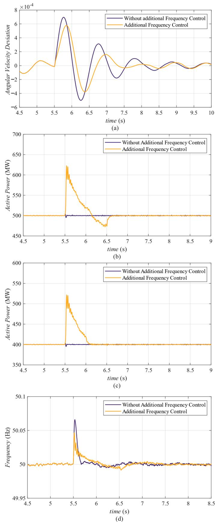
**Figure 7.** System response when the load at the sending end was removed. (a) Generator speed; (b) active power of line 3; (c) active power of line 4; (d) system frequency.
