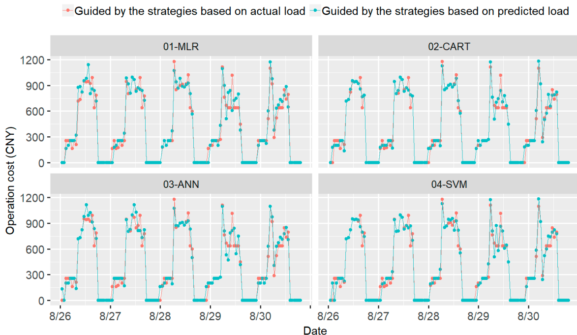
Figure 10. The hourly operation costs of the DHC system under different load conditions.
