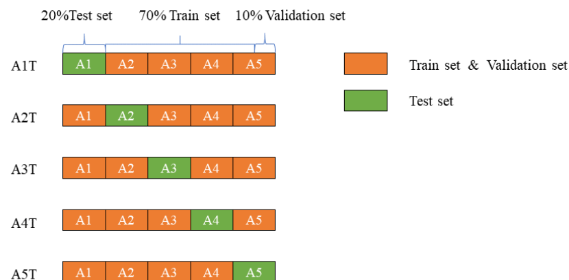
Figure 4. Schematic diagram of the dataset combination.
