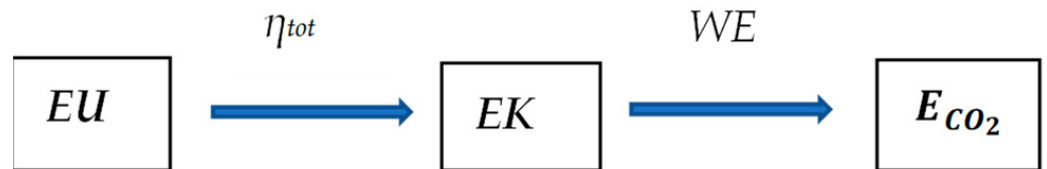
Figure 3. Schematic of transformation from EU to EK and E_{CO_2} indicators, where WE is CO_2 emission factor ( tCO_2/(m^2 \cdot year) ).
