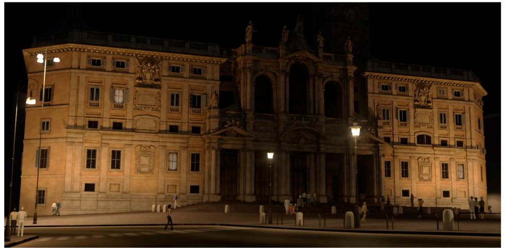
Figure 20. Visualization of the impact of street lighting with complementary flood illumination on the basilica model facade.
