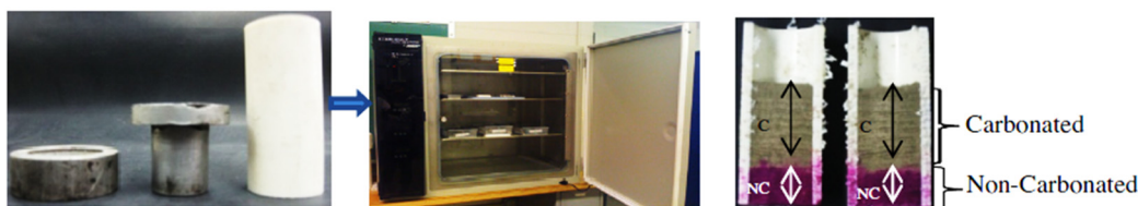
Figure 4. Procedure for the determination of carbonation depth [29]. Copyright 2015, with permission from Elsevier.
