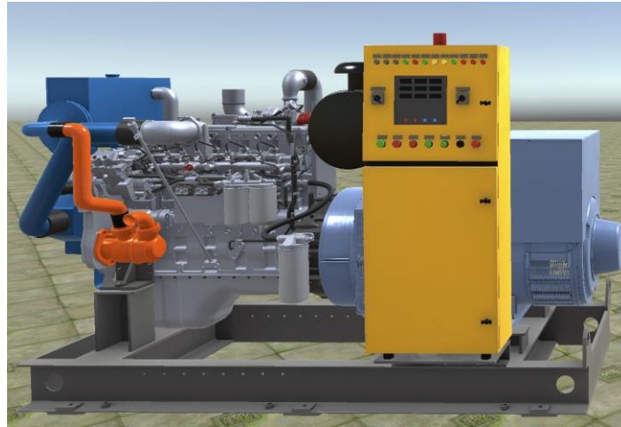
Figure 7. 3D model of diesel generator rendered in web interface.
