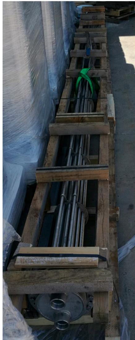
Figure 2. Downhole heat exchanger before installation in the geothermal well.
