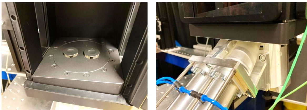
Figure 2. Optical chamber with the dual-intake valves from Engine B with up to 9 mm of valve lift (left) and 3D-printed dual-intake pipes reproducing the Engine B geometry (right).
