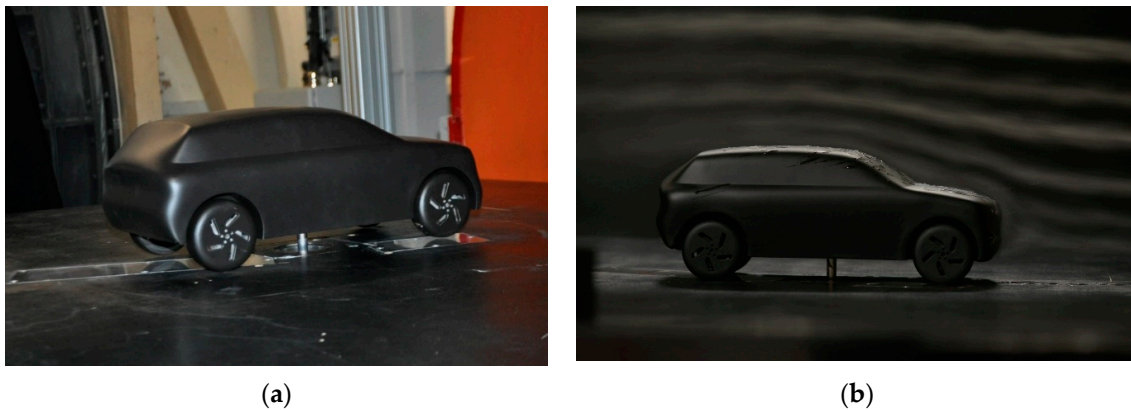
Figure 4. Test object: (a) generic SUV-class car, approximately 1:10 scale; (b) its exemplary flow visualization.
