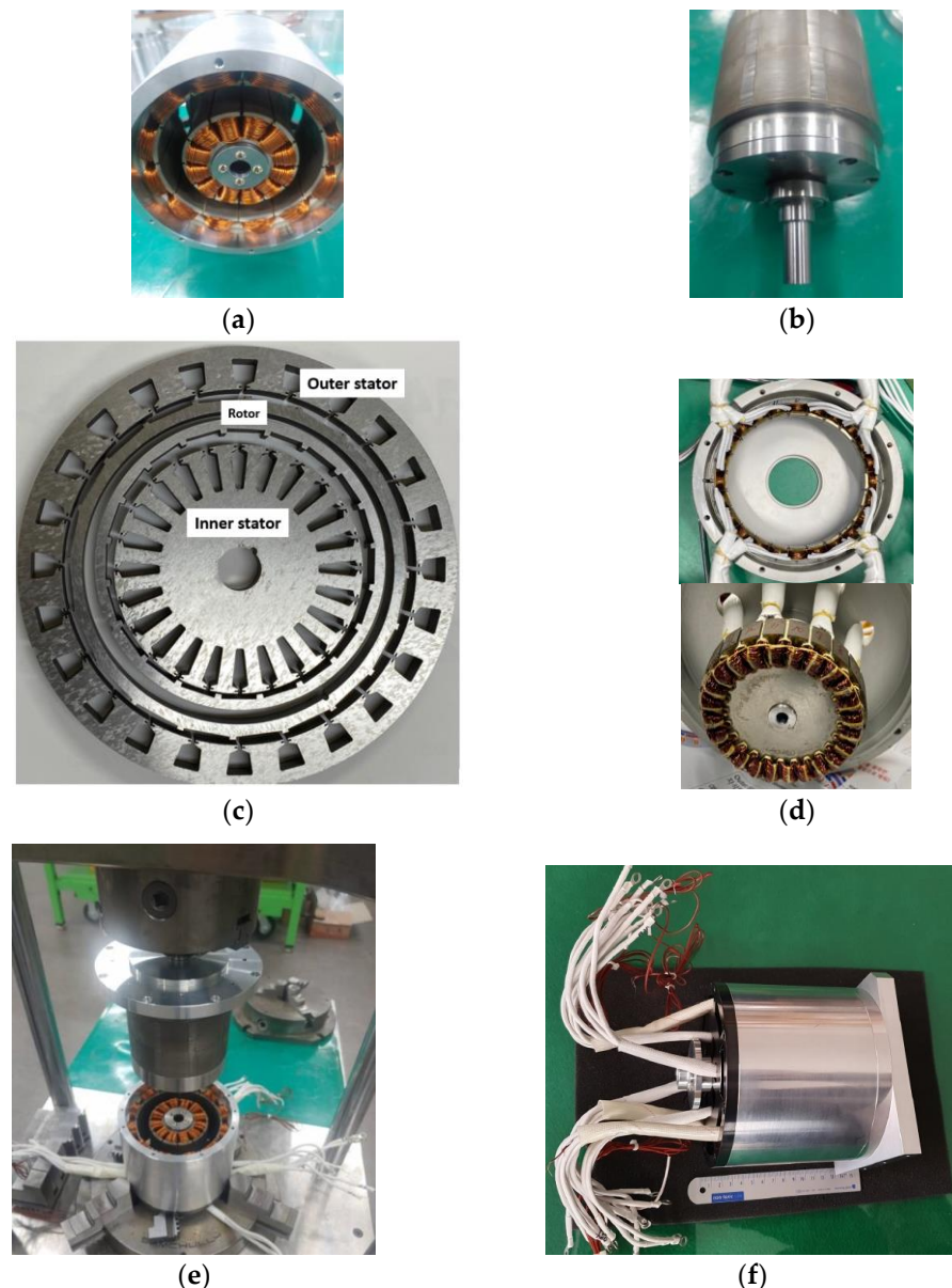
Figure 12. Prototype motor: (a) stator; (b) rotor; (c) stator and rotor cores; (d) winding connection; (e) rotor insertion process; (f) final assembly.
