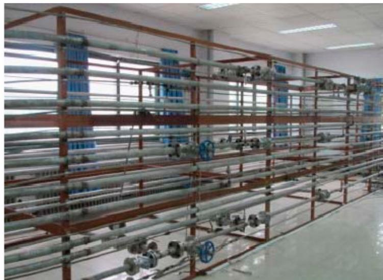
Figure 7. Diagram of the test loop with a 42 mm pipe diameter.
