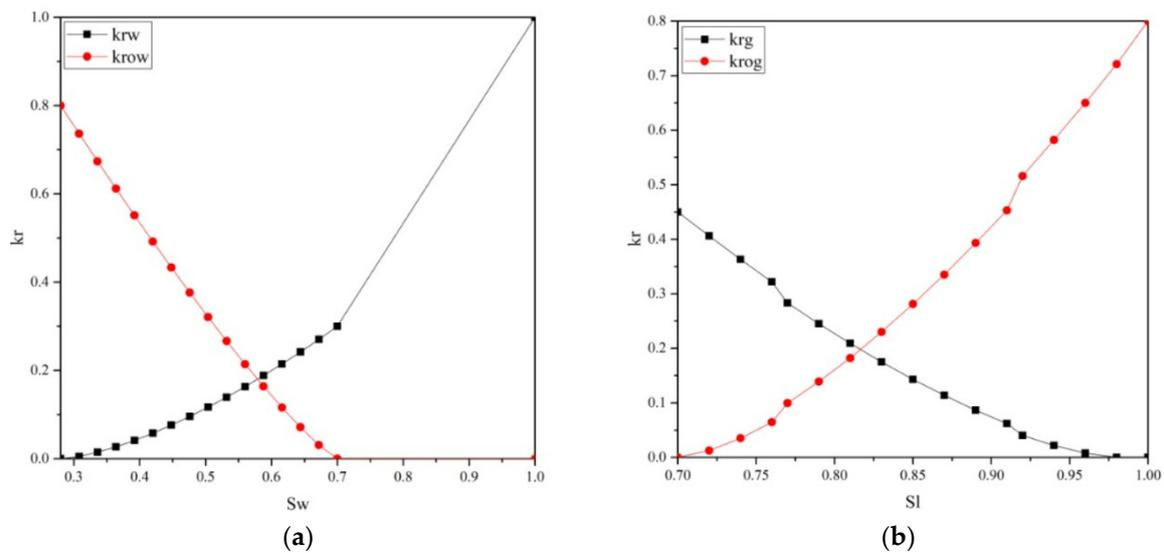
Figure 2. (a) Relative oil–water permeability curves; (b) Relative oil–gas permeability curves.
