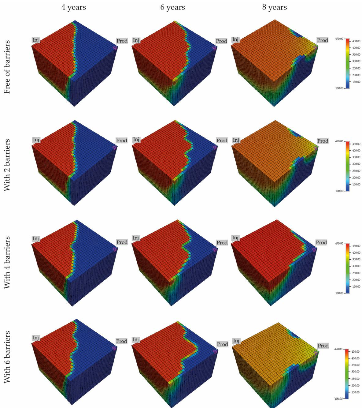
**Figure 8.** Temperature maps for the simulated cases at 4, 6, and 8 years.
