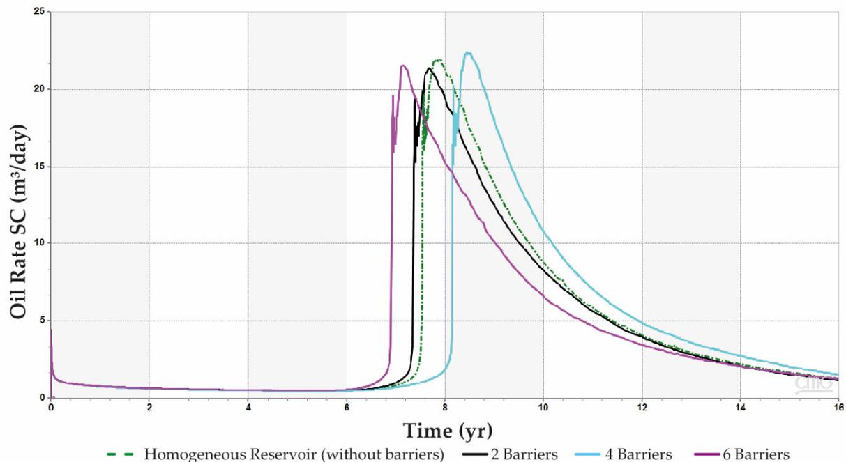
**Figure 6.** Oil flow rate as a function of 16-year project time.
