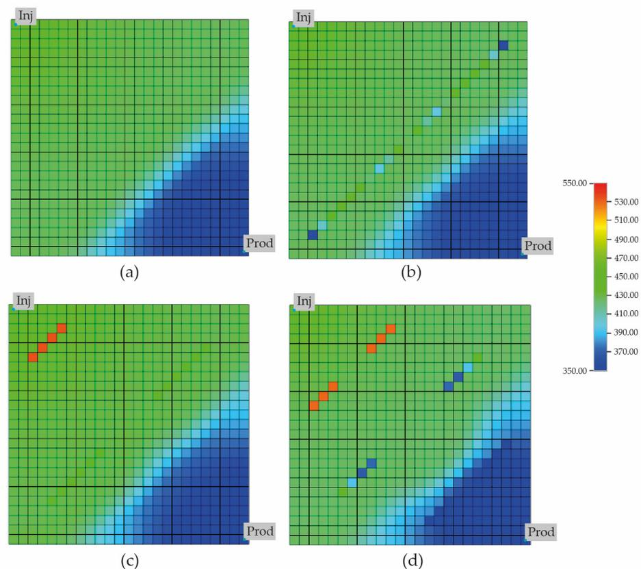
**Figure 9.** Pressure field at 5 years of steam injection for (a) barrier-free case; (b) 2 barriers; (c) 4 barriers; and (d) 6 barriers.
