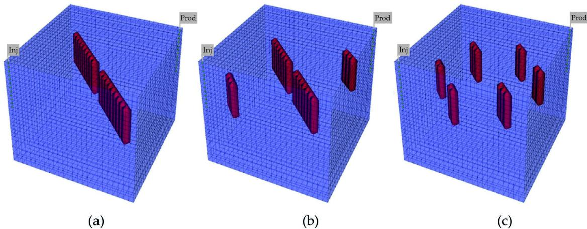
Figure 3. (a) Reservoir model with 2 barriers; (b) Reservoir model with 4 barriers; (c) Reservoir model with 6 barriers.
