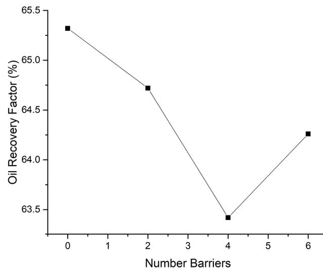
**Figure 5.** Recovery factor after 16 years of steam injection.
