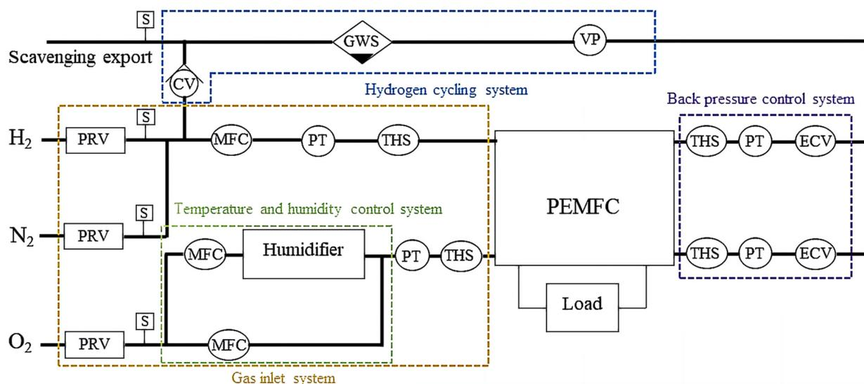
**Figure 2.** Schematic diagram of the gas control module.
