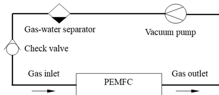
Figure 4. Diagram of the hydrogen cycle module.
