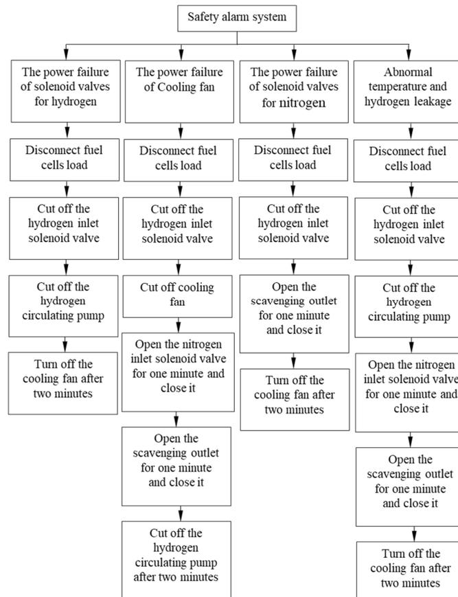
**Figure 6.** Flow chart of the safety alarm module.
