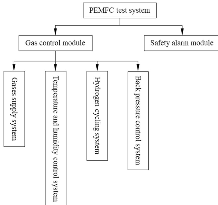
**Figure 1.** Basic composition diagram of the PEMFC test system.
