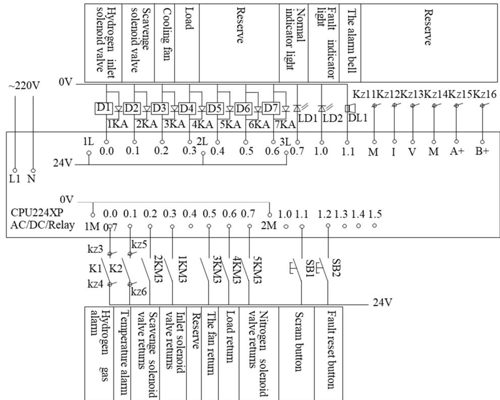
Figure 7. Main electrical connection diagram of the PLC.
