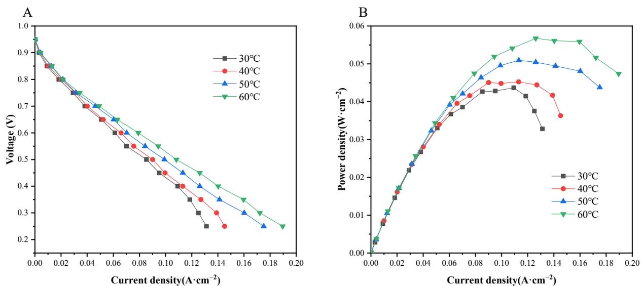
Figure 12. Fuel cell performance curves at different humidification temperatures. (A) Polarization curves and (B) power density curves.
