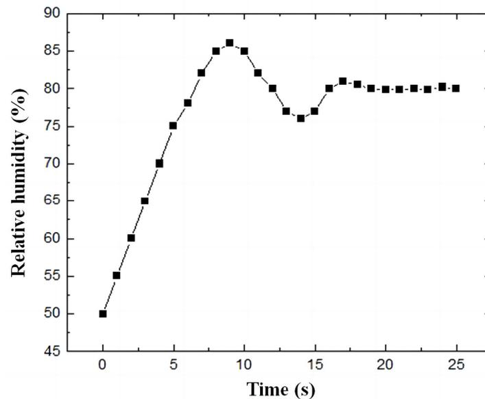
Figure 11. Variation curve of the relative humidity with time.
