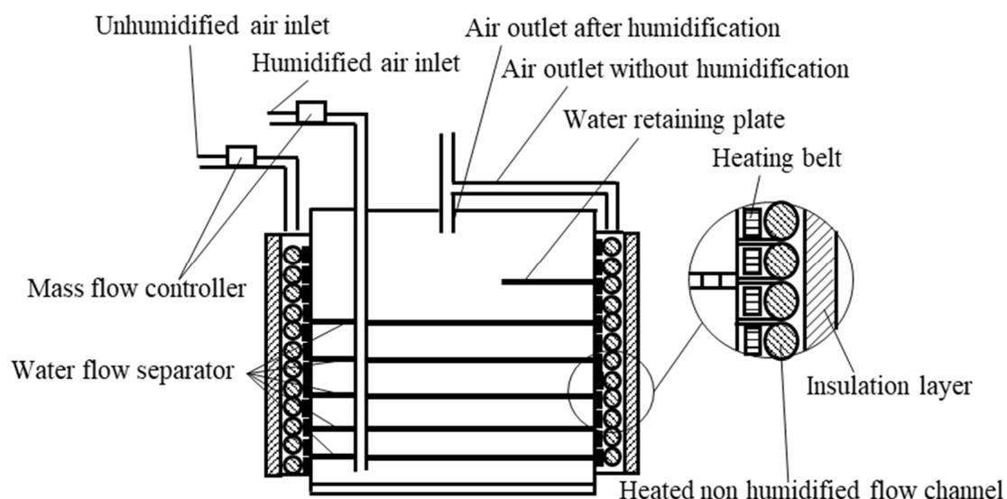
Figure 3. Section view of the humidifier.
