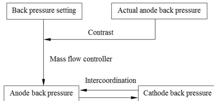
**Figure 5.** Flow chart of the back pressure control module.
