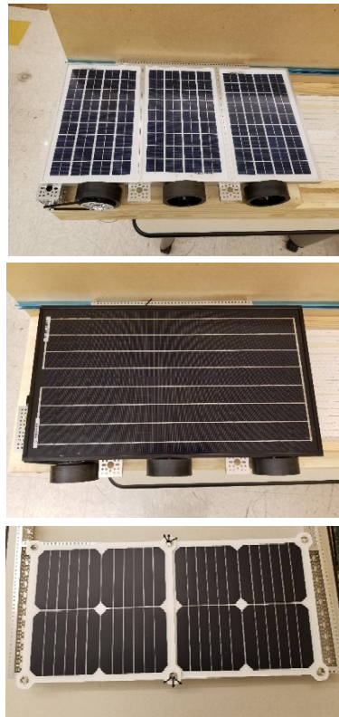
Figure 7. Three solar panel frames constructed for lab-scale prototype: Top to bottom: Three 10 W EcoWorthy ® , 30 W Renogy ® , 2–13 W SunKingdom ® .
