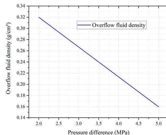
**Figure 11.** Influence of pressure difference on overflow fluid density.
