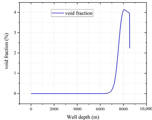
**Figure 7.** Void fraction diagram in annular space of Well Y.
