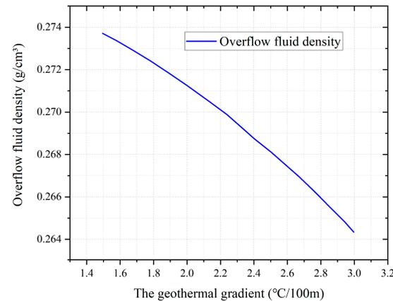
**Figure 10.** Influence of geothermal gradient on overflow fluid density.
