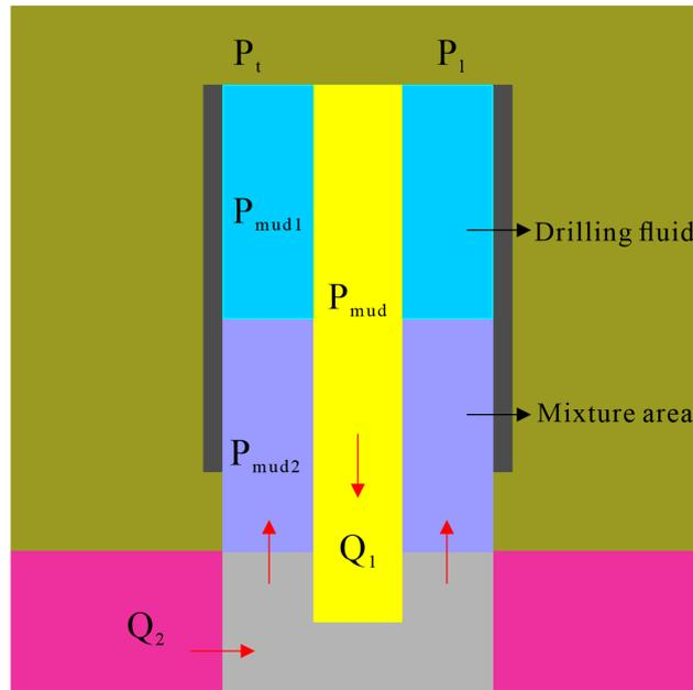
Figure 3. U-tube principle after air gas kick.
