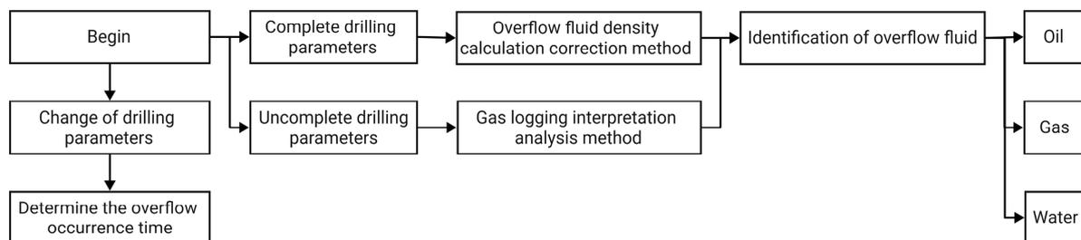
**Figure 6.** The process of identifying overflow fluid type.
