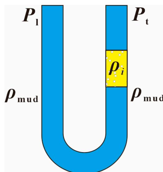
Figure 1. Schematic diagram of the U-tube principle.
