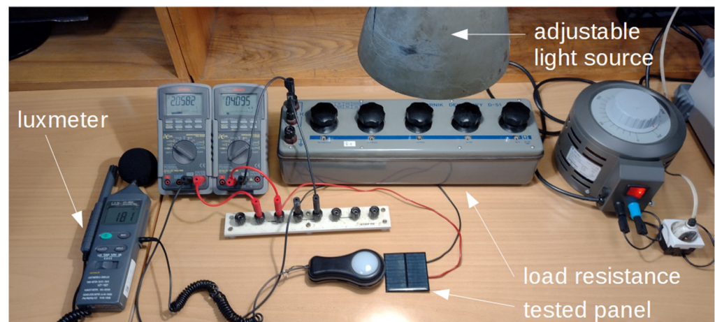
Figure 11. Measurement stand for determining the parameters of a solar cell.
