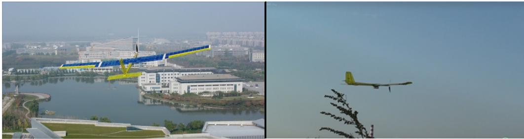
**Figure 13.** Empty aircraft flight verification and 4 kg payload flight verification.
