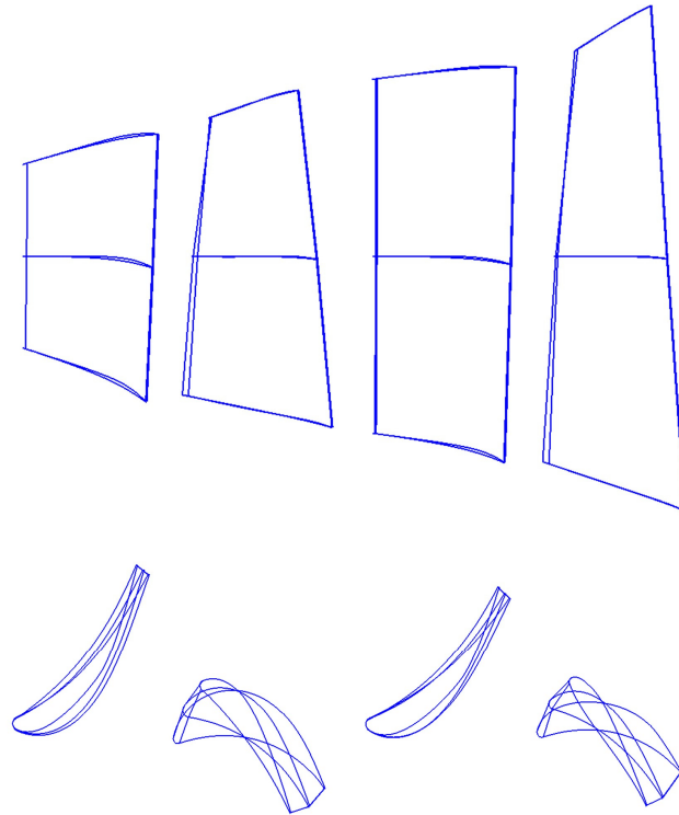
Figure 5. Three-dimensional blade geometry of the two-stage axial turbine.
