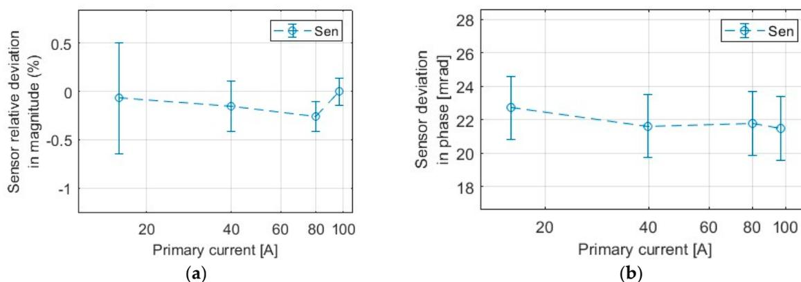
**Figure 3.** Uncertainty of the errors. (a) Uncertainty of the ratio error; (b) uncertainty of the phase error.
