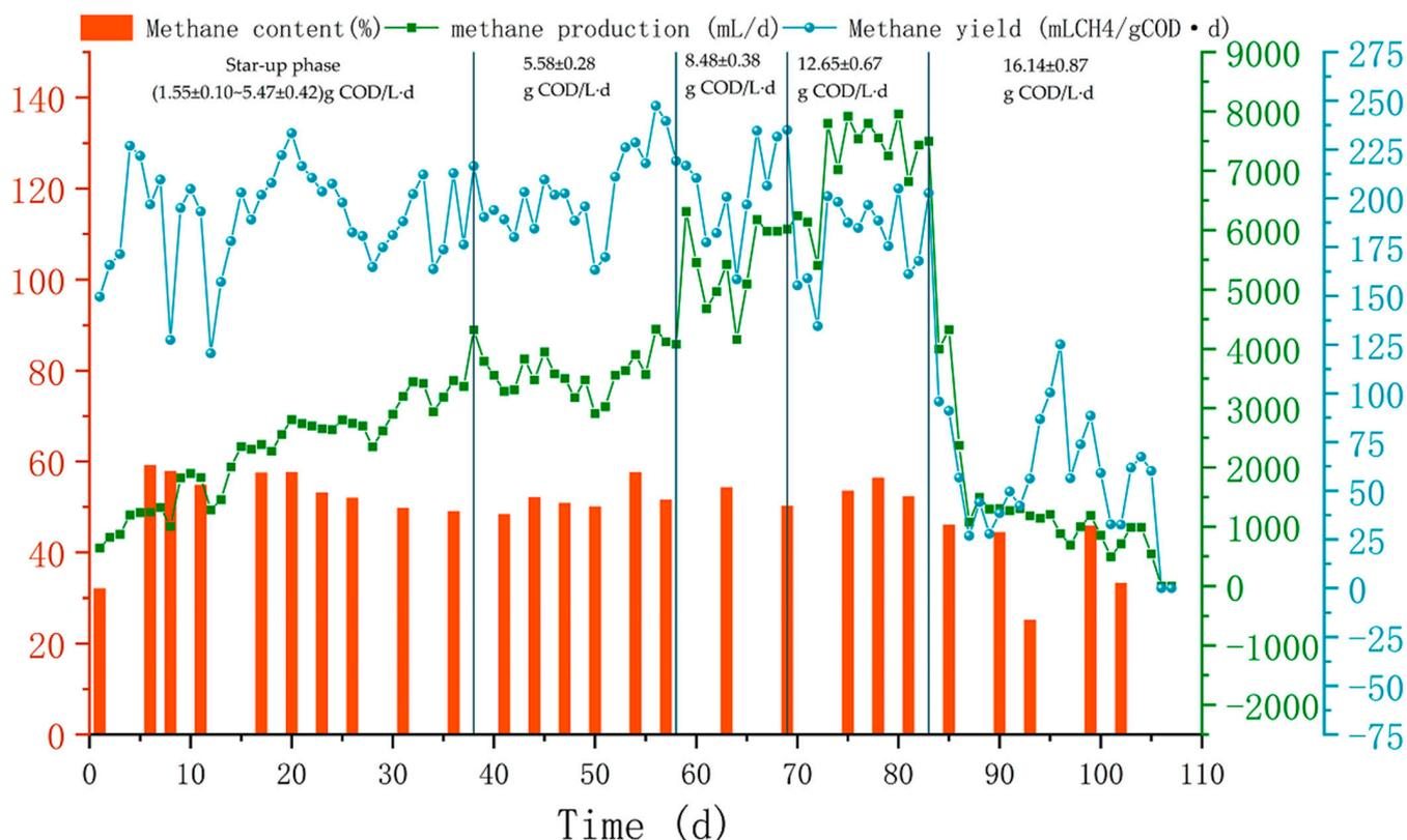
**Figure 3.** Methanogenic performance of EGSB reactor for treatment of CAW.
