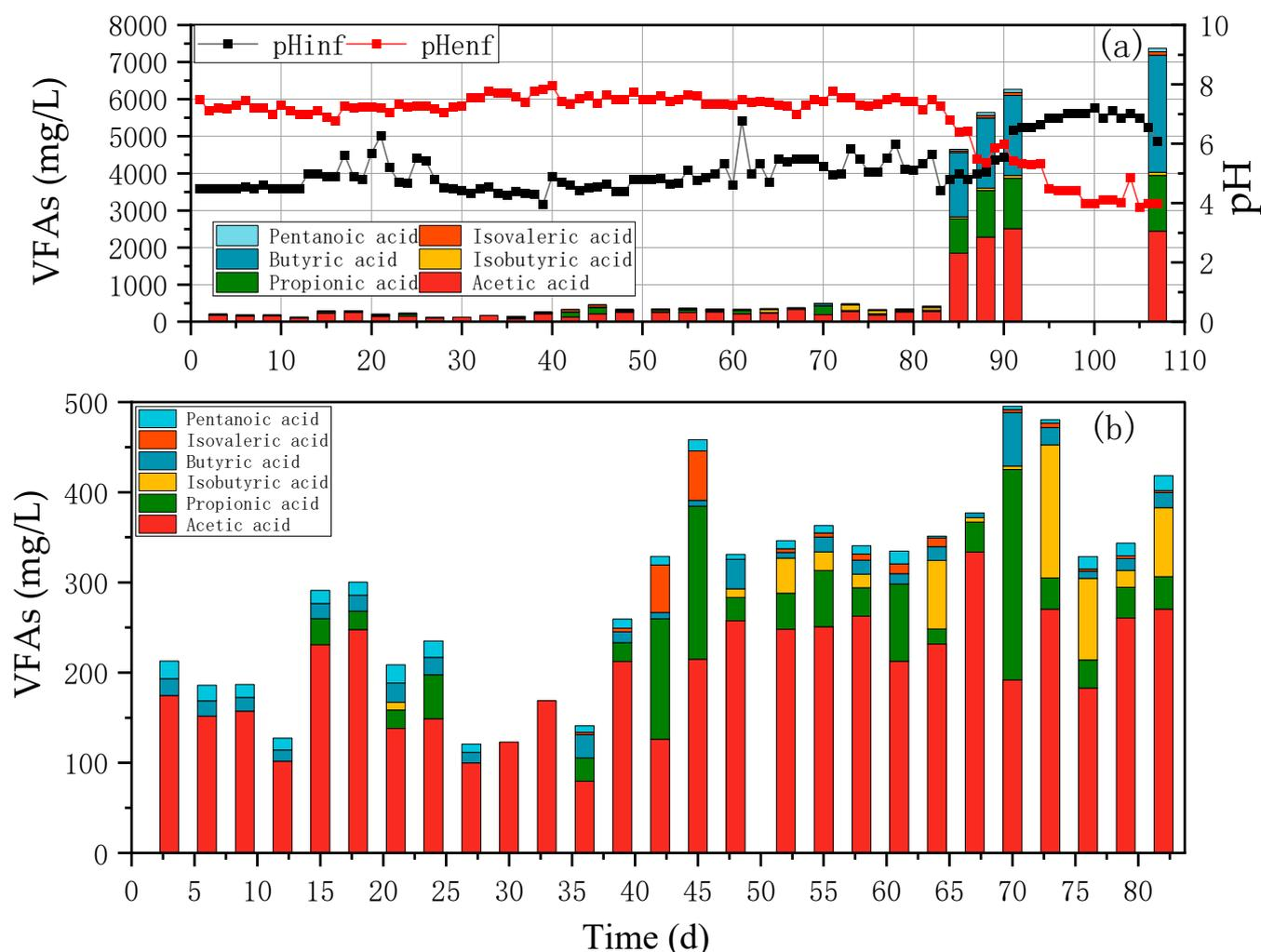
**Figure 5.** Variation in VFA content and pH in EGSB reactor effluent, where (b) is a magnified image from day 1 to day 83 in (a).
