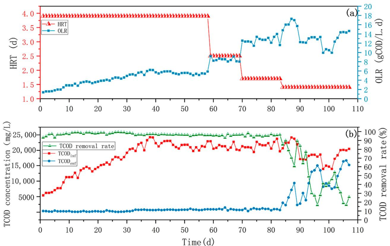
**Figure 2.** Organics removal of the EGSB system: OLR and HRT (a), and TCOD concentration and TCOD removal (b).
