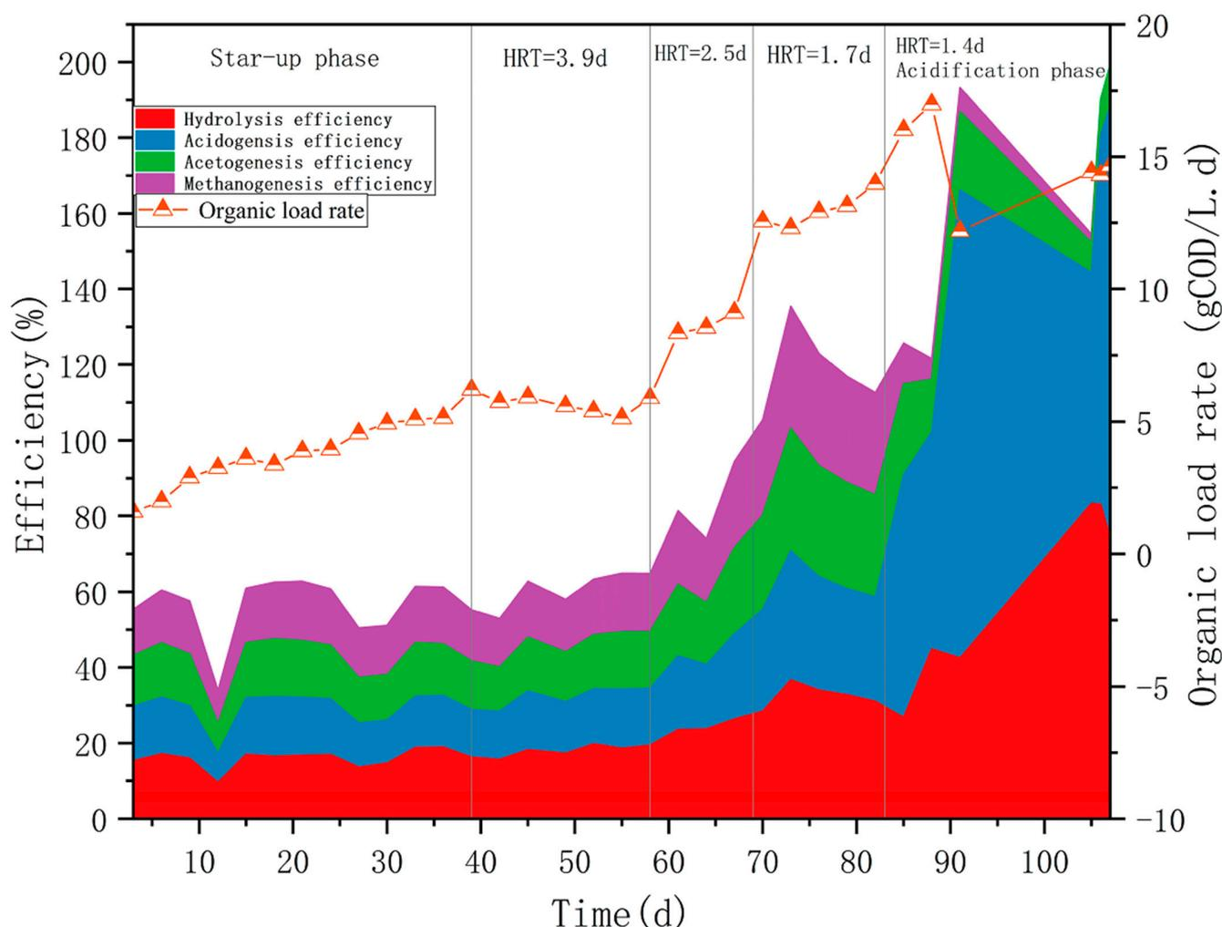
**Figure 6.** Four-stage efficiencies of EGSB system: hydrolysis, acidogenesis, acetogenesis, and methanogenesis.
