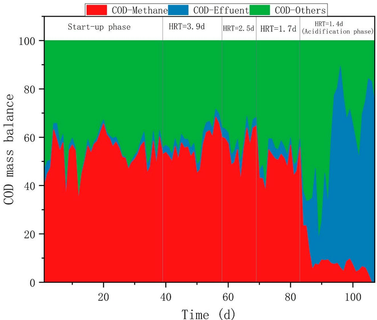
**Figure 4.** COD balance of EGSB reactor for treatment of CAW. COD–effluent: COD in the effluent, COD–others include COD–discharge (COD discharged as waste sludge) and COD–sludge accumulation (COD accumulated in the reactor), and COD–methane: COD converted to methane.
