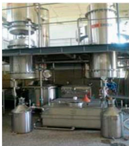
Figure 1. Presentation of the distillation process of lavender and/or oregano for the production of lavender and/or oregano oil, respectively.
