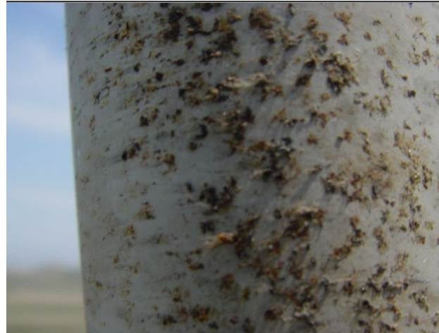
Figure 14. Contamination of insects on HAWT blade [154].
