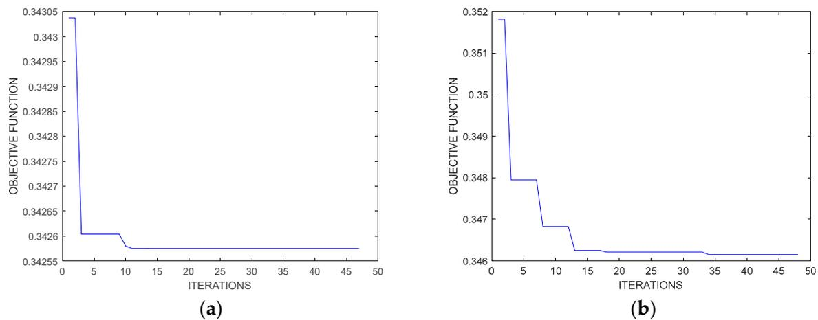
**Figure 15.** Evolution of the objective function in the 34-bar system for scenario 1 without THDv restriction (a) and scenario 2 with THDv restriction (b).
