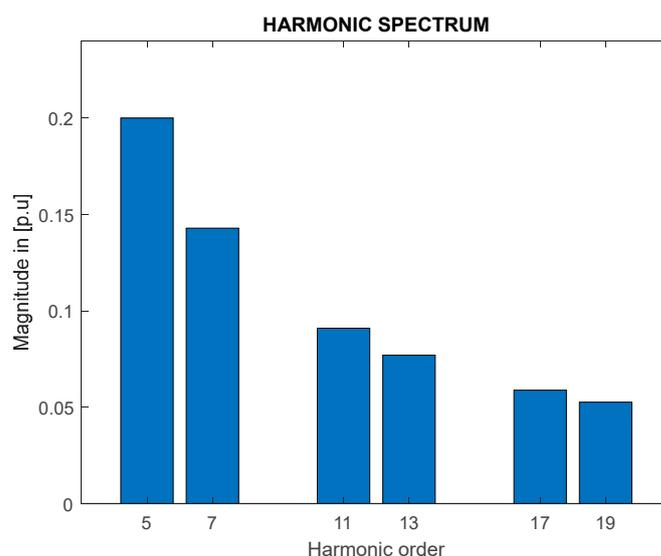
**Figure 1.** Typical harmonic spectrum of a 6-pulse converter.
