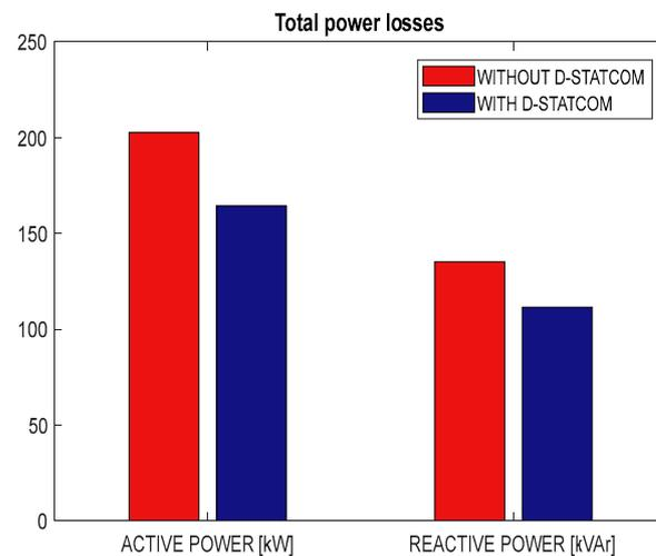
**Figure 7.** Power losses in scenario 2 for the 33-bar system.
