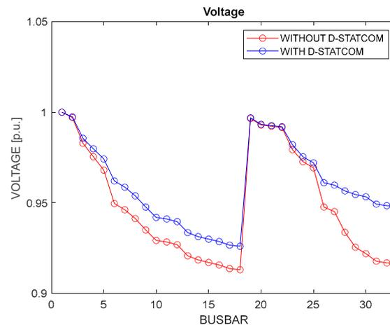
**Figure 4.** Voltage profile in scenario 1 for the 33-bar system.
