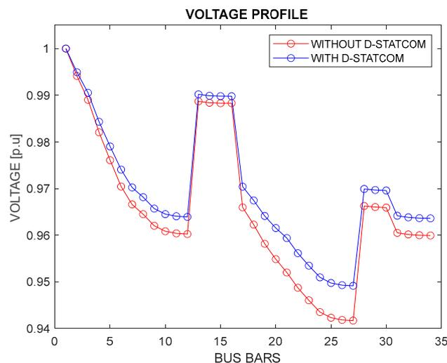
**Figure 10.** Voltage profile in scenario 1 for the 34-bar system.
