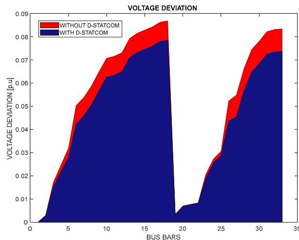
**Figure 6.** Voltage deviation in scenario 2 for the 33-bar system.
