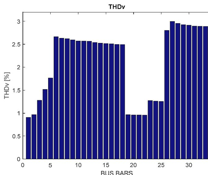
Figure 8. Voltage THD in scenario 2 for the 33-bar system.
