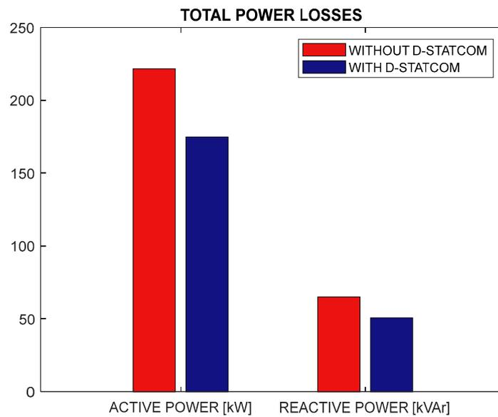
Figure 13. Power losses in scenario 2 for the 34-bar system.
