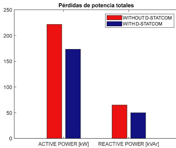
Figure 11. Power losses in scenario 1 for the 34-bar system.
