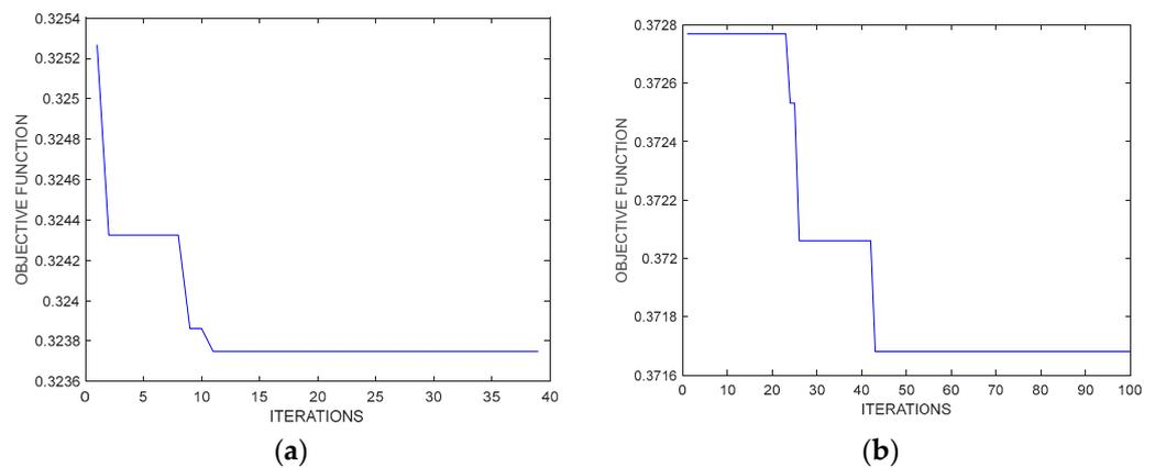
**Figure 9.** Evolution of the objective function for scenario 1 without THDv restriction (a) and scenario 2 with THDv restriction (b).
