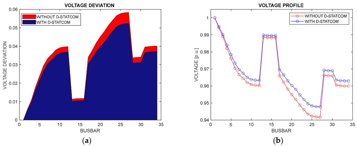
Figure 12. Voltage deviation in scenario 2 for the 34-bar system (a). Voltage profile in scenario 2 for the 34-bar system (b).
